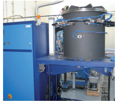
Hot filament Chemical Vapour Deposition reactor for diamond deposition
