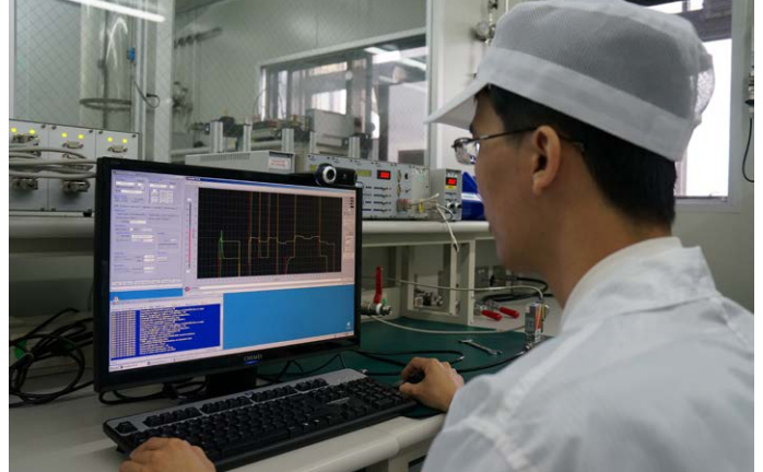
Service Engineer, optimizing (PID) controller settings
